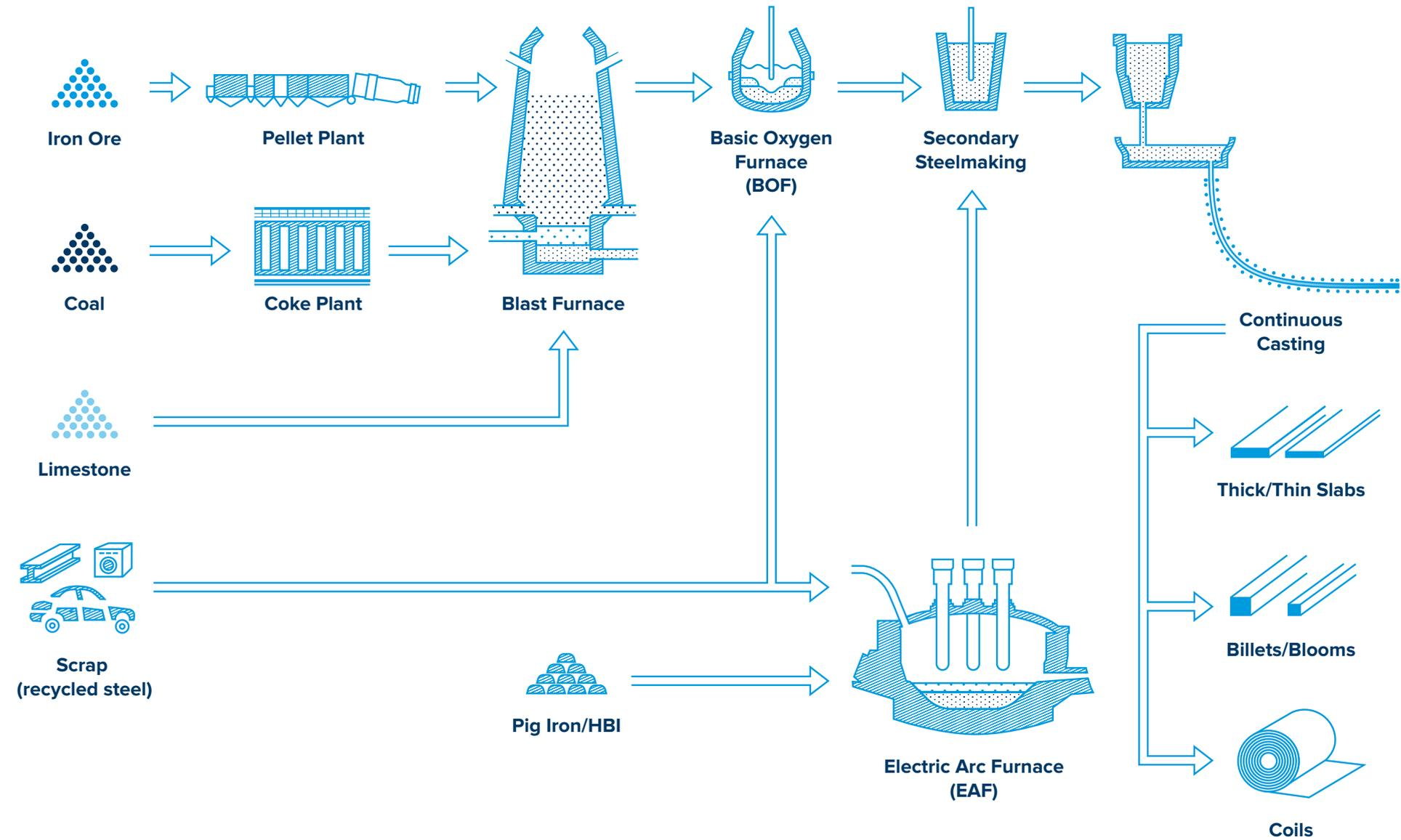
*Integrated steel mill (BOF) vs mini mill (EAF) process and equipment requirements*
